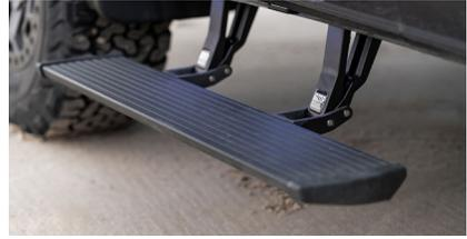
Figure 6-16. Power Step driver side
