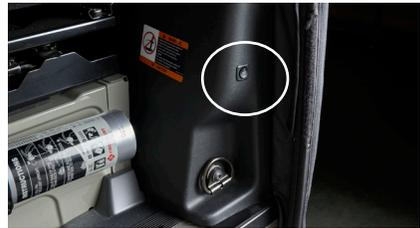
Figure 6-18. Power Step override switch near the slider door
