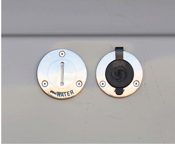
Figure 4-4. Exterior Water Connections
