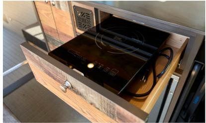
*Figure 5-21. Portable induction stove storage drawer*
