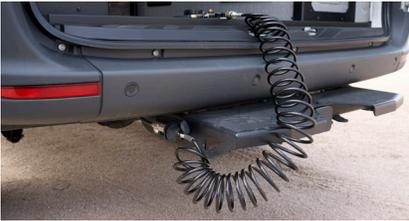
Figure 6-13. Rear Air Hose Connection
