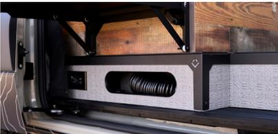
Figure 5-14. Power outlet and storage location
