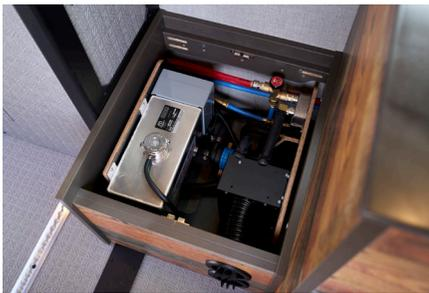
Figure 5-10. Furnace access under driver's side jump seat
