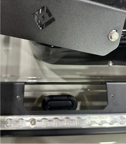
A cable port has been added to the ceiling panel in the Connectivity Cabinet for ease of installation of cell boosters or satellite antennas like Starlink. To open the cover pull down on the cover, the SCANSTRUT pass-thru is directly above this cable port.
