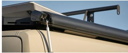
*Figure 6-6. Awning crank rod attachment*
