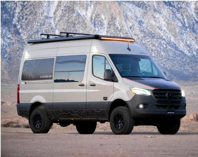
*Figure 6-3. Exterior lighting — Light Bar with Amber Setting, Side Lights, and Fog Lights*
