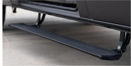
Figure 6-17. Power Step passenger side
