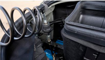
Figure 6-15. Under Hood Air Hose Connection
