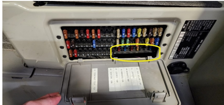
2018 and older vans heater fuse location. Drivers seat base
