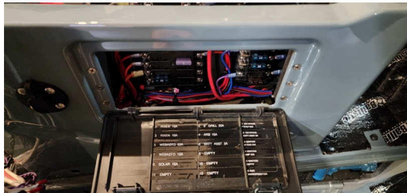
2019 and newer heater fuse location. Passenger seat base.
