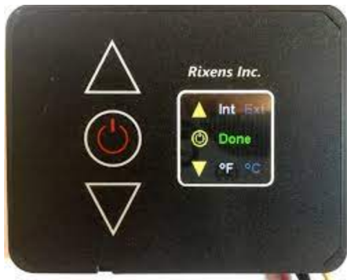
Heated floor temperature controller. Only vans with a heated floor system
