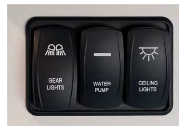
Figure 5-6. Switch Control Panel
