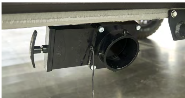
Figure 4-5. Grey Water Tank Drain
