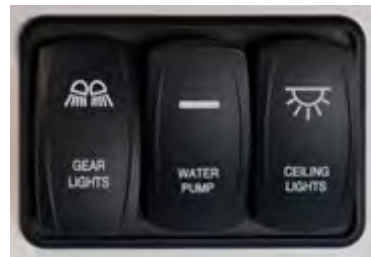
Figure 4-1. Upper Cabinet Switch Control Panel
