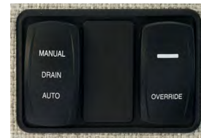
Figure 4-6. Shower Drain Switches
