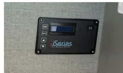
Figure 4-3. Tank Level Monitor
