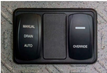
Figure 4-6. Shower Drain Switches
