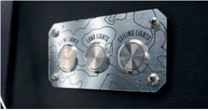
Figure 5-16. Scene Lights, Load Lights, and Ceiling Lights Push Buttons, located next to sliding door
