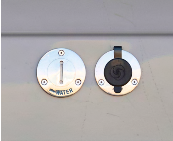
Figure 4-4. Exterior Water Connections
