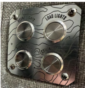
Figure 5-19. Scene Light, Load Lights, Gear Lights, and Ceiling Lights
