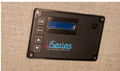
Figure 4-3. Tank Level Monitor
